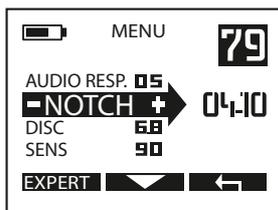
Notch complements discrimination: it enables a "window" of targets to be rejected whereas discrimination rejects all targets below a selected threshold.
