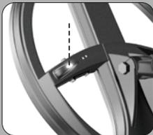
The LED on the coil gives 20 long, successive flashes to indicate that it is waking up and recalibrating.
